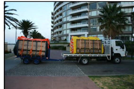
Picture shows 2 bundles each containing 400m of ADSB fitted with a 1m 270gsm non woven. The Curtain is fitted with ballast chain and floats and the skirt is furlled to the floats. The curtain bundle is contained within a laced cover which is fitted with lifting straps.
