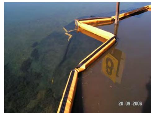
Model ADSB fitted with a PP8 2m skirt containing heavy sediments in a tidal waterway
