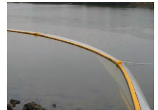
Model ADSB Fitted with PET100 High Strength skirt deployed in a tidal waterway
